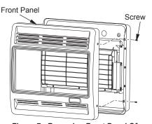
Figure 7 - Removing Front Panel Of Heater
